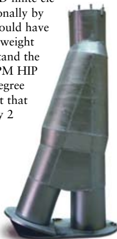
Wye-piece in duplex stainless steel made by Sandvik Powdermet. The angle between the legs is 15 degrees and maximum wall thickness 80 mm (weight 2 tonnes).
