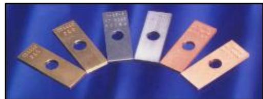
The simplicity of the measurement offered by the corrosion coupon is such that the coupon technique forms the baseline method of measurement in many corrosion monitoring programs.
