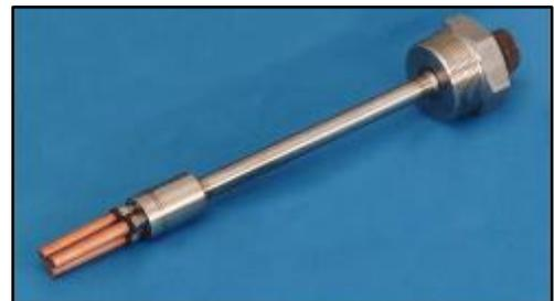
The advantage of the LPR technique is that the measurement of corrosion rate is made instantaneously. This is a more powerful tool than either coupons or ER where the fundamental measurement is metal loss and where some period of exposure is required to determine corrosion rate. The disadvantage to the LPR
